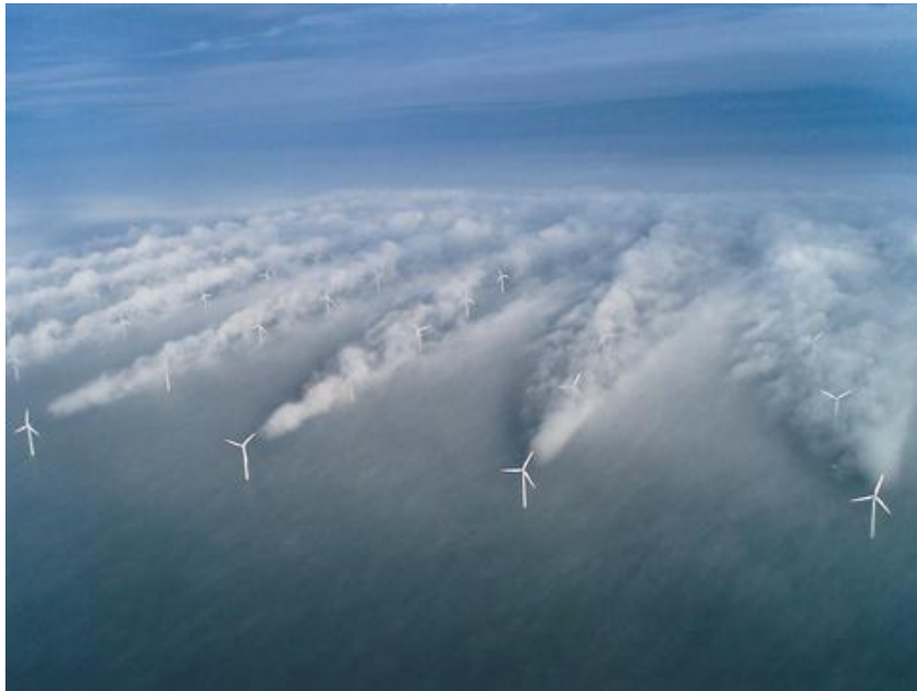
Figure 7: Wake Turbulence Behind Turbines Illustrated by Sea Fog.
