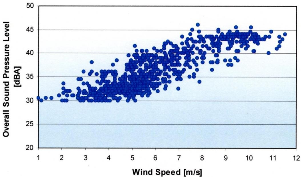
Converting back to the 10 metre wind speed, the turbine noise was out of compliance for virtually all of the time that the wind speed was above about 5 metres/second.
