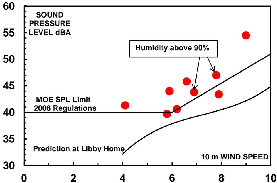
Figure 1: Measured sound pressure level (SPL) as a function of 10m wind speed.
